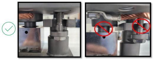
TOP PLATE VIEW: When aligned correctly, the pin is centered in the top plate. Note that this top view may be obstructed when the mount is under support legs.
