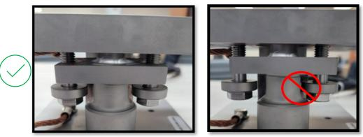
SIDE VIEW: When properly aligned, liftoff bolts will be centered in the machined center post cavity.
